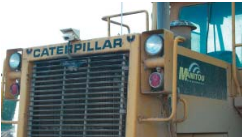
A camera is mounted to the chassis (above) and a monitor is mounted in the cab (left).
