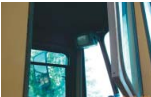
A camera is mounted to the chassis (above) and a monitor is mounted in the cab (left).
