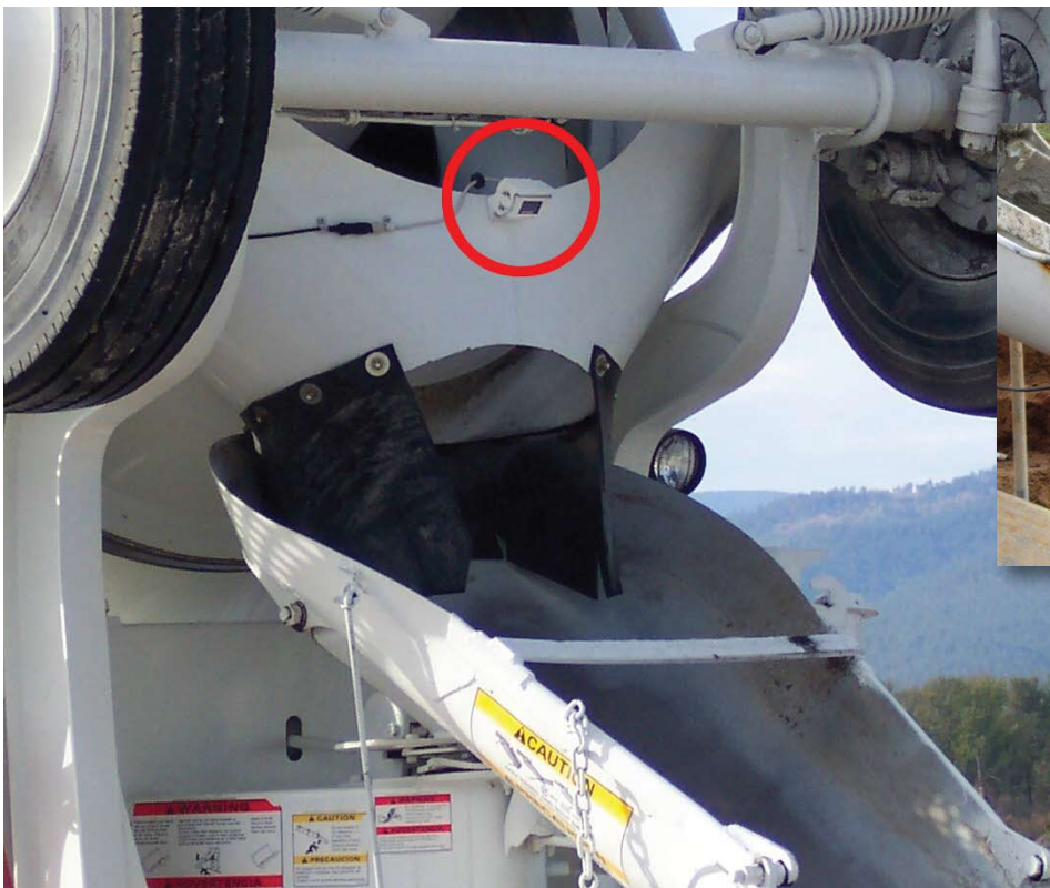
This camera mounted on the chute allows Vulcan's drivers to stay clear of concrete pumps.
