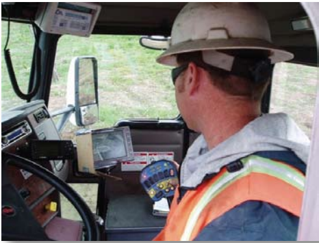
Video technologies can be used like another mirror, and allow drivers to monitor conditions while staying safely out of harm's way. Shown is a driver for Vulcan Materials Company monitoring concrete coming down the chute of his ready-mix truck.
