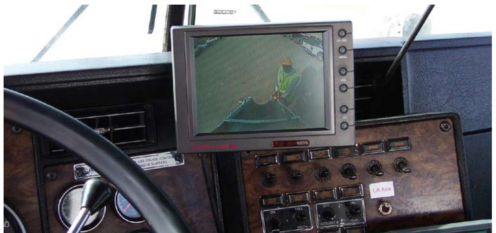
With the use of camera technology, drivers for Vulcan Materials can see directly behind the truck and monitor the material flowing down the chute from the safety of the cab.
